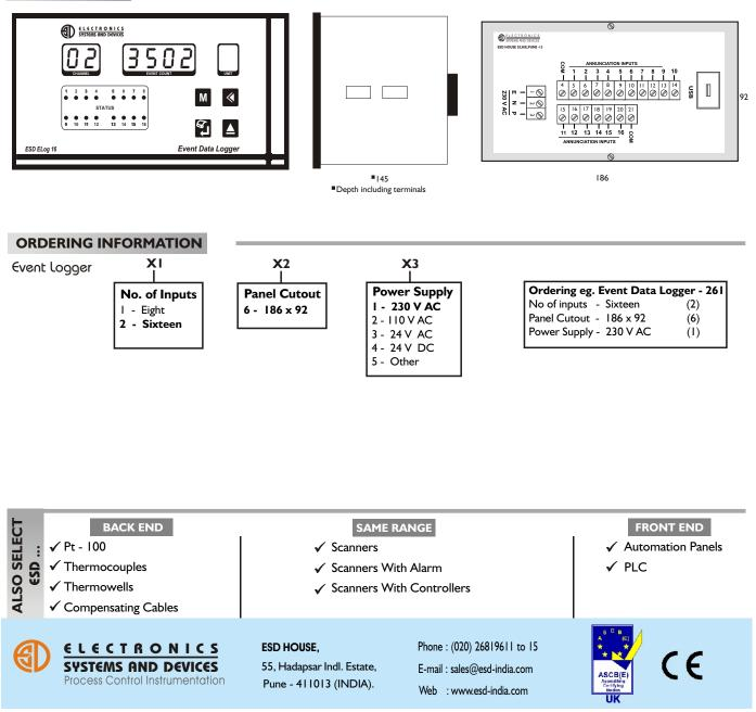
Unspecified dimensions are in mm. Photos not to the scale. Due to continuous development above details are likely to change.
