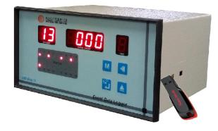
User can connect a hooter through relay for audio alarm. Facility to connect external 'Test & Accept' push buttons is available. Multiple flashing rates are provided for differentiating various fault types.
