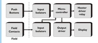
The single chip microcontroller of the Data Logger series continuously monitors all the connected inputs. If a fault occurs in any of the inputs, then it is detected by the CPU. According to the nature of the fault, the CPU will decide the status of the
