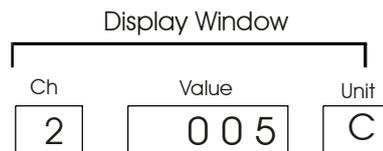
After the last channel unit displays following message and will go to Automode.
