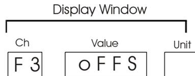
When user press enter key unit will display following message, using increment and shift keys user can set offset value in between - 9.9 to + 9.9 for particular channel.
